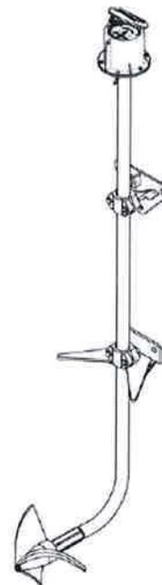
A commercially available package that includes a reverse propeller meter and trash-shedding fixed vane, plus flow straighteners, is available from RSA.
